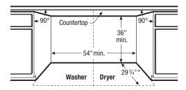
Side-by-Side Units in Under-Counter Installation Can be installed with standard countertop and/or cabinetry.
